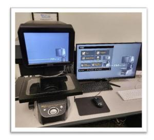
This Mitutoyo CMM is a high-speed automatic touch technology CMM which can measure hundreds of dimensions per hour.
